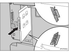
**7** Hold the handle, and carefully pull out the printer board halfway.
