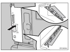
Lock the printer board with the two screws you removed in stepA.
