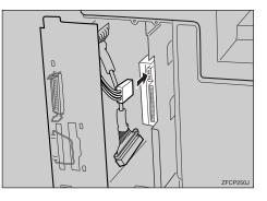
Connect the connector to the Printer Hard Disk.
