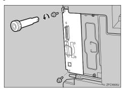
**5** Remove the two screws locking the hard disk drive cover next to the printer board.
