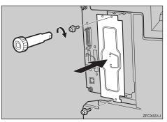
Align the printer board with the top and bottom rails in the printer, and then insert the printer board slowly until it stops.
