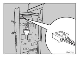
**9** Connect the connector to the printer board.
