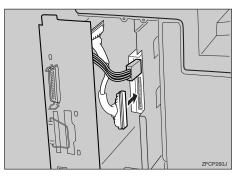
Lock the Printer Hard Disk cover with the two screws you removed in step **5**.
